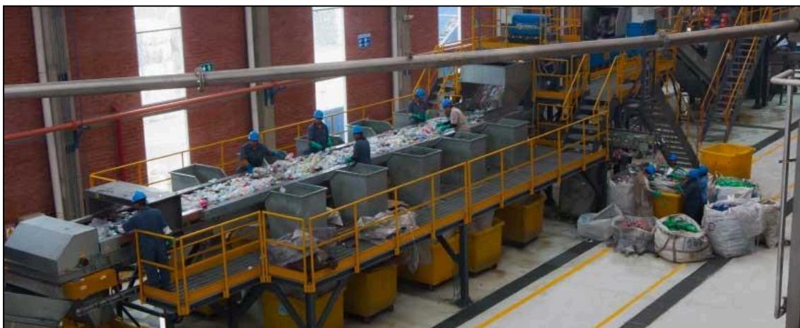
Figure 4: Hand picking section in bottle-to-flake PET bottle recycling unit of ENKADOR
