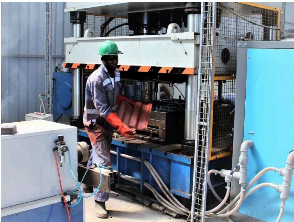
Figure 6 The press can produce 6 tiles at once.
