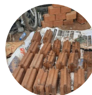
Prototype of interlocking bricks
